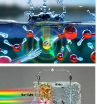
FPMD+GW simulations of photoanodes (WO<sub>3</sub>) for water splitting. Gerosa et al. Nature
