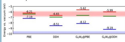
Band offsets and flat-band potentials computed using G<sub>0</sub>W<sub>0</sub> calculations (WEST code) starting from FPMD trajectories and wavefunctions generated with hybrid functionals
